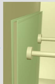
The panes are pressed together
