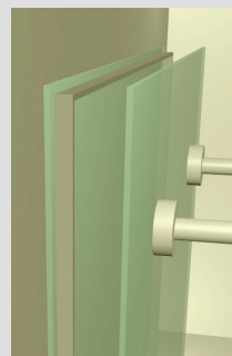
Argon gas is flooded into a chamber
